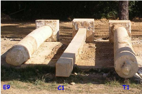
Fig.14. Piles after extraction.
